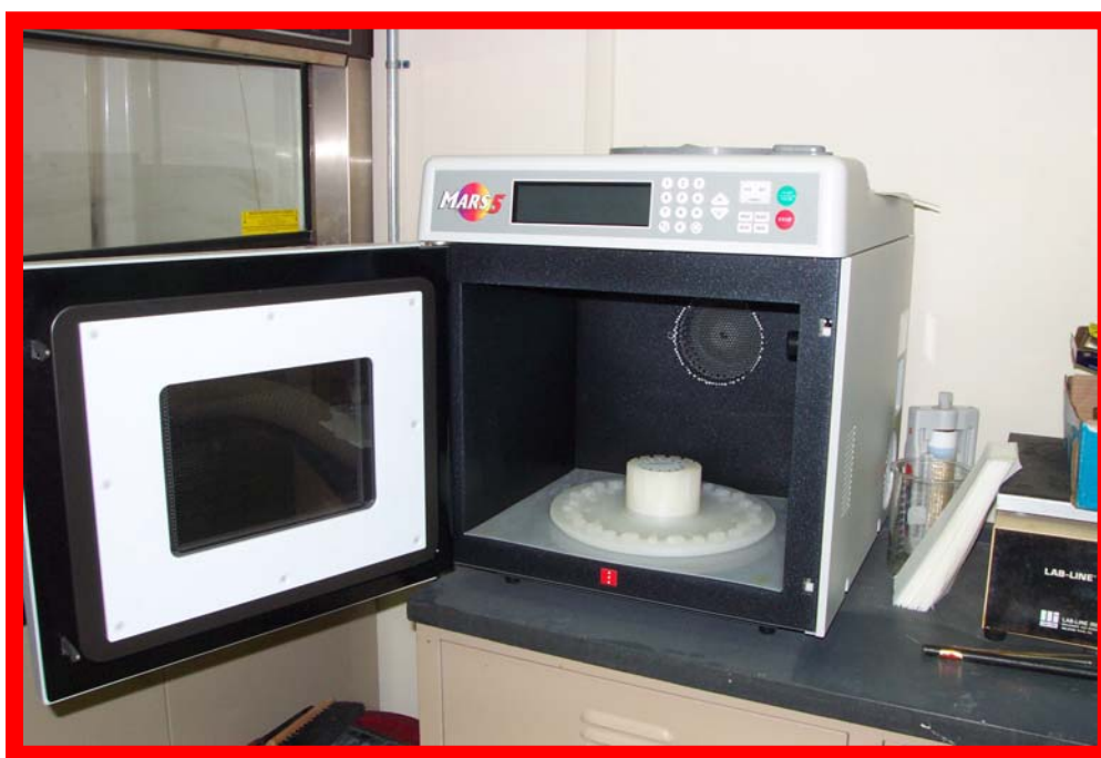
Figure 2. Microwave reaction chamber for hydrothermal experiments.
