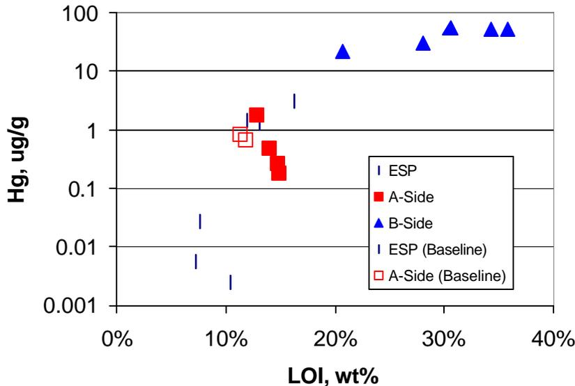
Figure 2. Mercury and LOI contents of ash from Gaston long-term PAC testing at 1.5 lb/MMacf injection rate.
