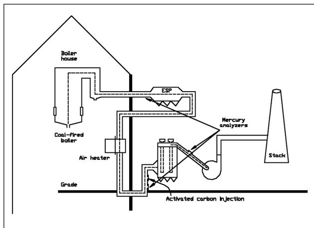
**Figure 1.** Flow schematic of Gaston Unit 3, showing injection and measurement locations.
