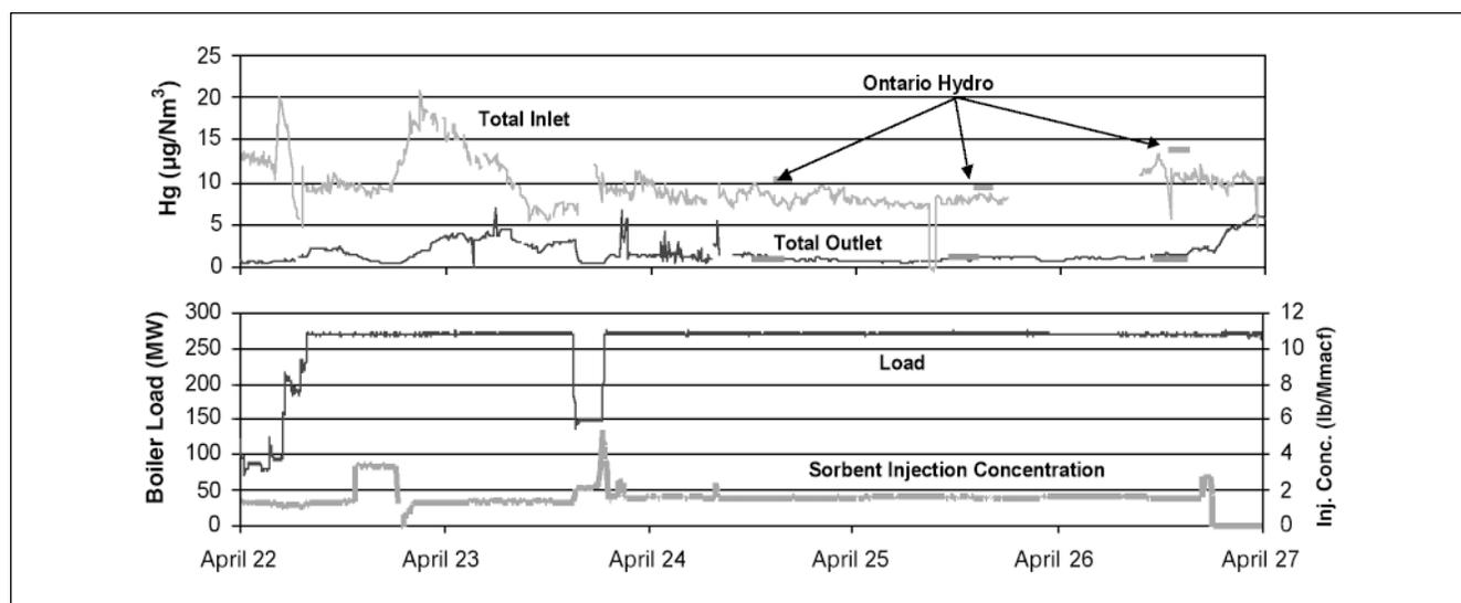
**Figure 7.** Inlet and outlet COHPAC Hg concentrations, boiler load, and PAC injection concentration during long-term tests, April 2001.
