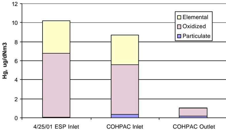
Figure 1. Mercury in flue gas at Gaston Station during long-term PAC testing at 1.5 lb/MMacf injection rate as measured by Ontario Hydro method.
