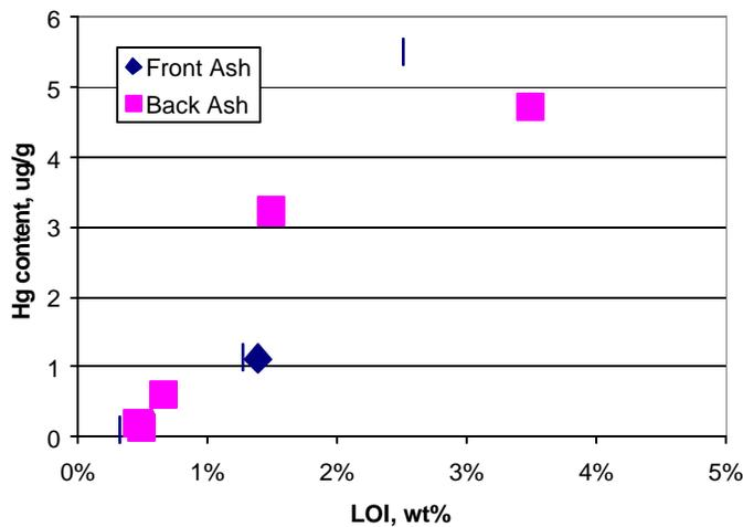
Figure 4. Mercury and LOI contents of ash from Pleasant Prairie long-term PAC testing at 0-10 lb/MMacf injection rate.
