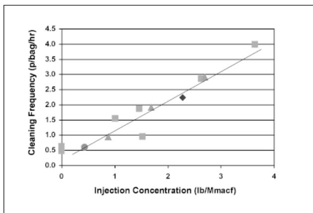
**Figure 6.** COHPAC cleaning frequency in pulses/bag/hr as a function of PAC injection concentration. Measurements made during parametric tests, March 2001.
