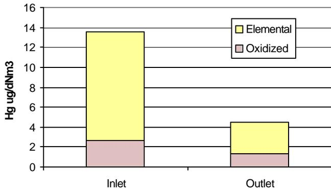
Figure 3. Mercury in flue gas (gas-phase only) at Pleasant Prairie during long-term PAC testing at 10 lb/MMacf injection rate as measured by S-CEM.
