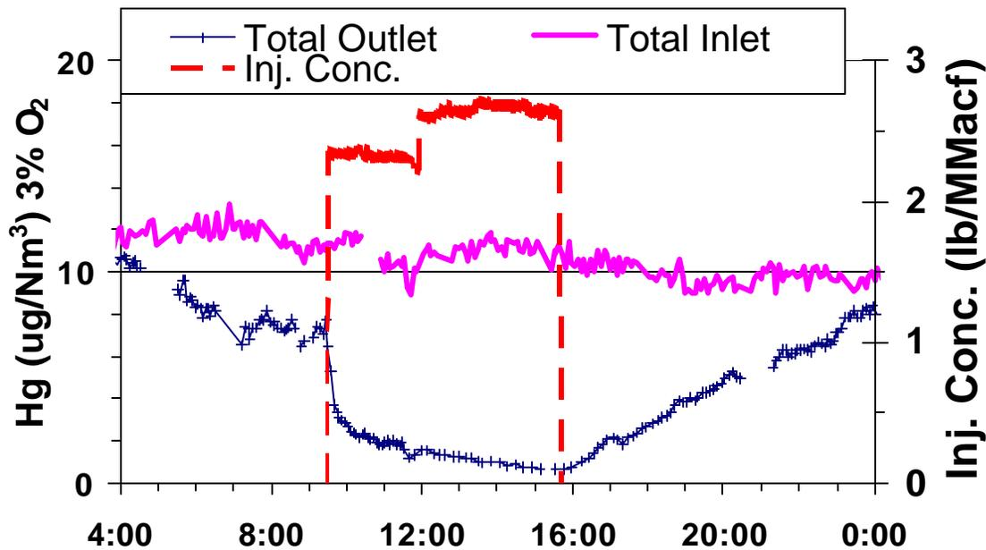
**Figure 3. Mercury removal trends across COHPAC as a function of PAC injection concentrations. Measurements made during parametric tests, March 2001.**
