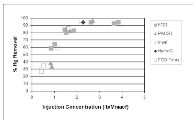
**Figure 5.** The Hg removal trends across COHPAC as a function of PAC injection concentrations. Measurements made during parametric tests, March 2001.
