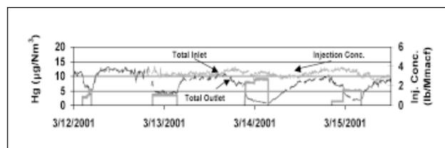
**Figure 4.** S-CEM Hg measurements during the first week of parametric tests with Norit Darco FGD PAC.
