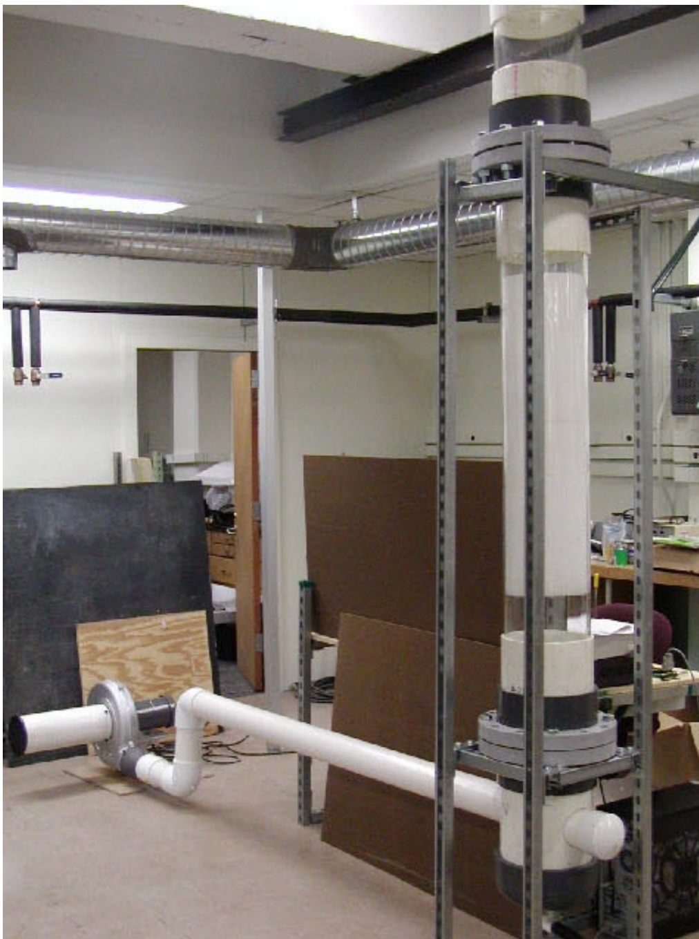
Figure 41 Assembled View of Diffusion Tower
