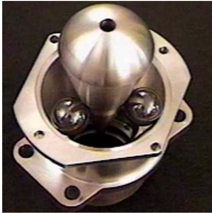
Figure 7. Sealing plug in its inactive position supported on the three locking balls positioned in the lower shell.
