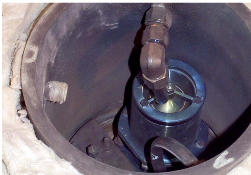
Figure 20. Top of P2 following run 15. A very small amount of ash and/or refractory material can be seen resting where the sealing plug meets the upper shell. The pulse tube is positioned over the top of P2.
