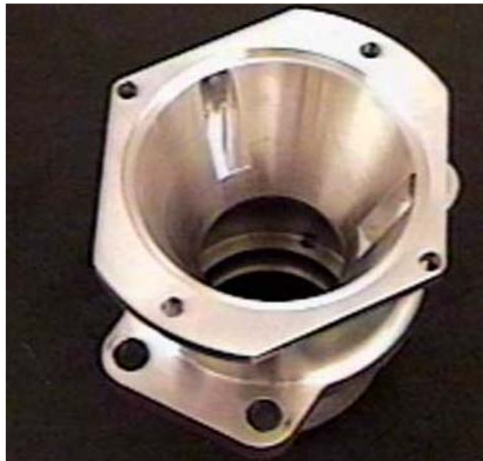
Figure 8. Lower shell showing the vertical channels used to maintain the 120° spacing of the three locking balls during activation.
