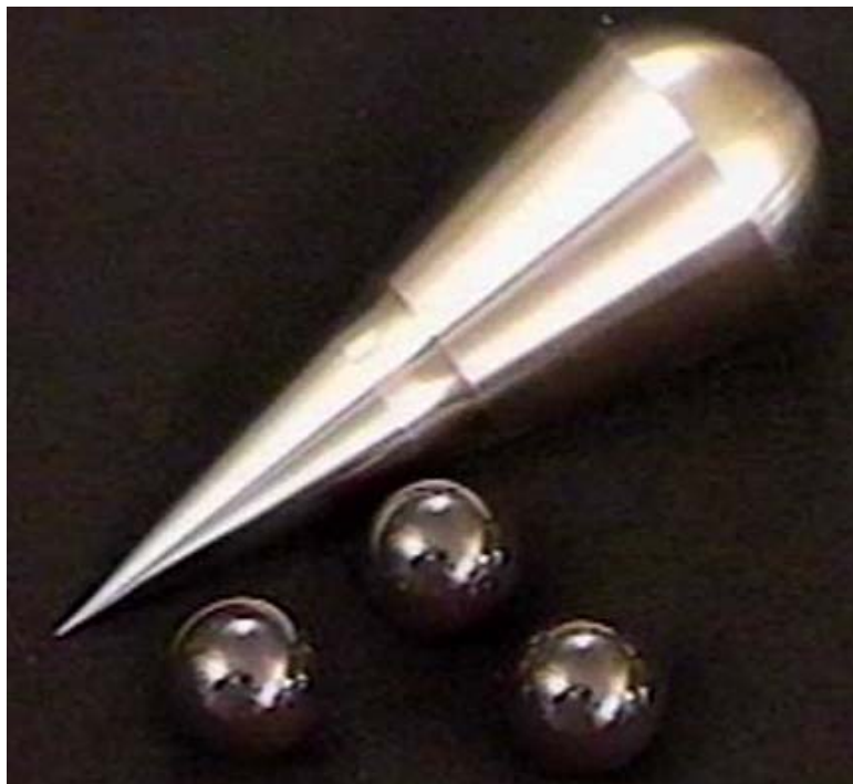
Figure 6. P2 sealing plug and locking balls.
