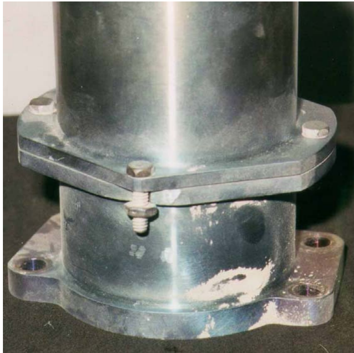
Figure 29. Condition of the SGD after run 15. The small ash deposit visible on the outside of the shell near the bottom of the SGD may provided a source of ash particles that could have been reentrained by the reverse-gas cleaning pulses.
