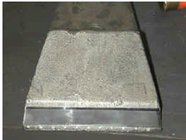
Figure 6g – FM wear resistant component in bucket lip for The Robbins Group—frontal view. The FM has a shiny appearance compared to the dull bucket lip.
