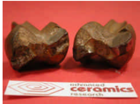
Figure 6f – WC(3%)Co/WC(25%)Co buttons fabricated for drilling tests (left), failed drill bits with FM inserts.
