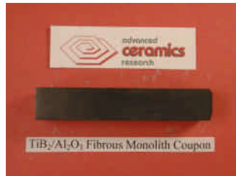
Figure 2a. 3" x 0.5 x 0.5" ZrB 2 /BN (left) and TiB 2 /Al 2 O 3 Fibrous Monolith coupons fabricated for testing and evaluation. The photo at left shows a 0.25" thick slice cut from the FM coupon.
