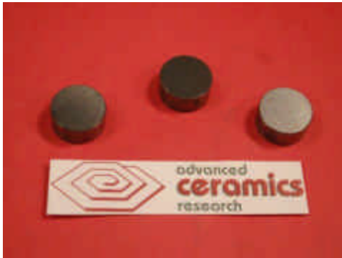
Figure 6f – WC(3%)Co/WC(25%)Co buttons fabricated for drilling tests (left), failed drill bits with FM inserts.
