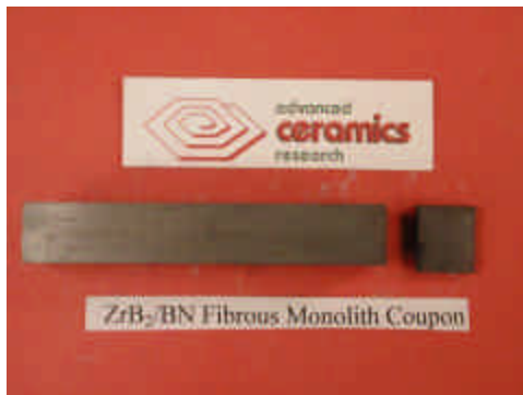
Figure 2a. 3" x 0.5 x 0.5" ZrB 2 /BN (left) and TiB 2 /Al 2 O 3 Fibrous Monolith coupons fabricated for testing and evaluation. The photo at left shows a 0.25" thick slice cut from the FM coupon.
