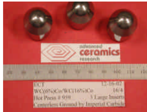
Figure 6c – Hot pressed WC-Co(6%)/WC-Co(16%) FM drill bit inserts before (left) and after (right) centerless grinding.
