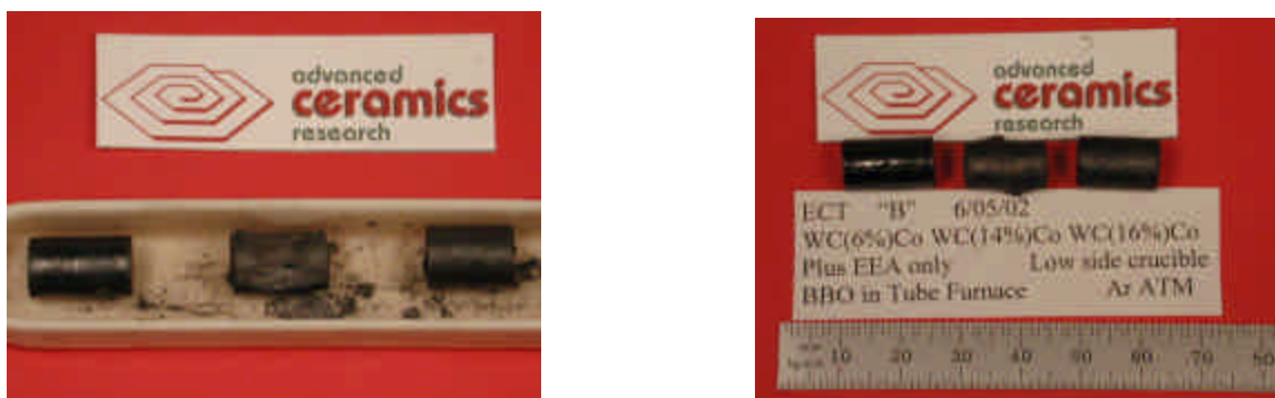
Figure 3d – WC-Co monolithic and FM test samples processed using binder removal profile “A” (left) and “B” (right) in a 3” diameter tube furnace under a flowing Ar atmosphere.
