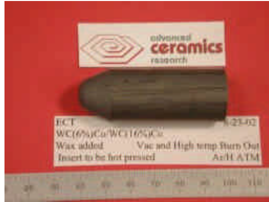
Figure 6b. WC-Co FM green drill bit insert for fabrication of hot pressed field test prototypes.
