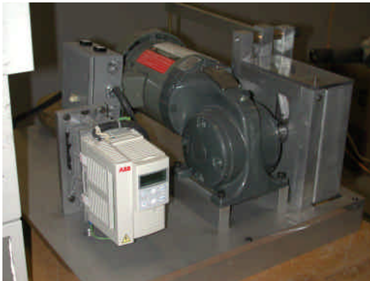
Figure 5a – High stress abrasion testing machine.
