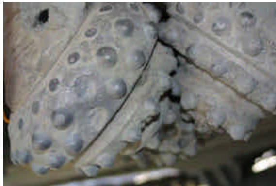
Figure 6e – Two of six drill bit inserts tested in the Iron Range of Minnesota shown on the roller cone to the left. The location can be identified as the two missing inserts.
