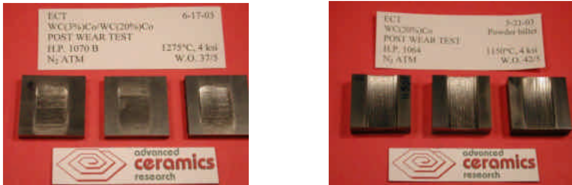
Figure 5b – Typical high stress abrasion wear tested samples, WC(3%)Co/WC(20%)Co FM left and WC(20%)Co powder coupon right.
