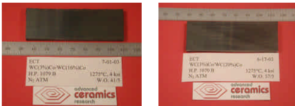
Figure 2c – Representative coupons fabricated with 82.5% core WC(3%)Co/ 17.5% shell WC(16%)Co on the left and 82.5% core WC(3%)Co/ 17.5% shell WC(20%)Co on the right
