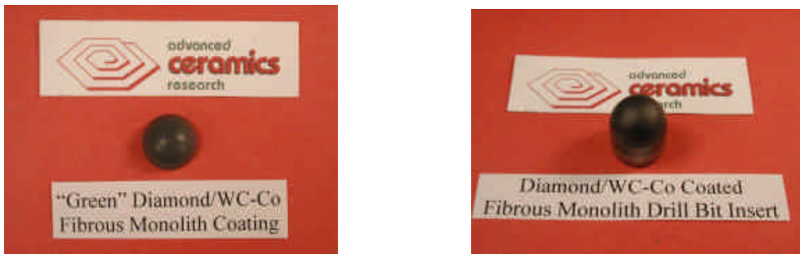
Figure 2b. Diamond/WC-Co Fibrous Monolith coating (left) and a consolidated Diamond WC-Co coating on a 3/8" WC oil drill bit insert.
