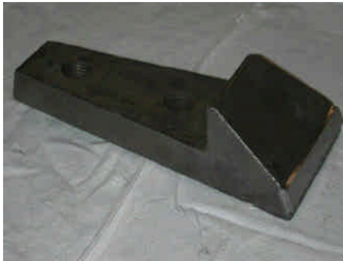
Figure 7a — Bucket lip provided by The Robbins Group for field testing of wear plate insert. Wear plate insert appears at the broad front edge of the bucket lip.
