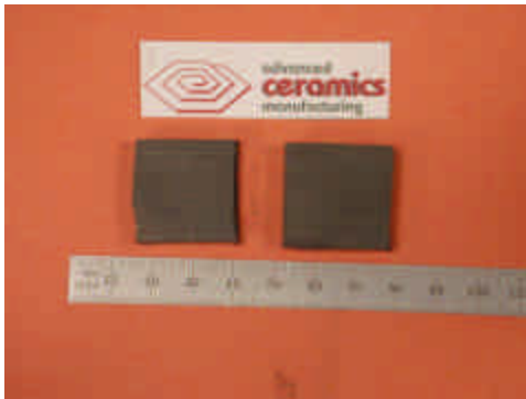
Figure 3a – WC-Co(6%)/Co FM test sample before (left) and after (right) binder removal in vacuum ( 10^{-3} torr) with a heating rate of 0.5 °C/minute to a set point of 500 °C.
