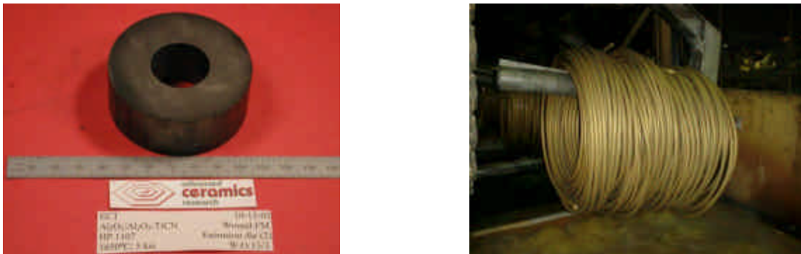
Figure 4c – Al 2 O 3 / Al 2 O 3 -TiCN FM extrusion die prior to machining (left) and approximately 1200 feet of 1” extruded brass rod (right).
