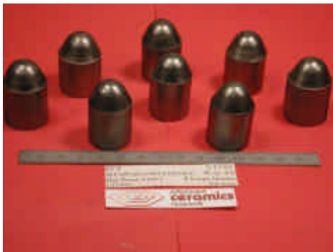
Figure 6c – Hot pressed WC-Co(6%)/WC-Co(16%) FM drill bit inserts before (left) and after (right) centerless grinding.
