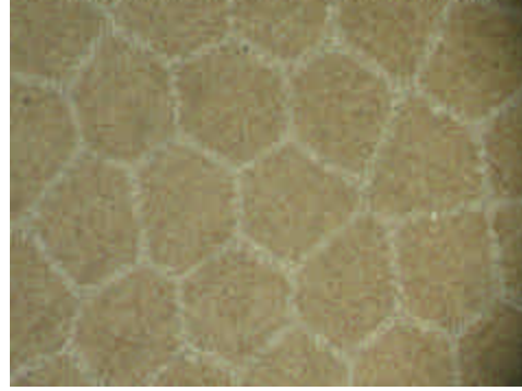
Figure 6d – Cross section of hot pressed WC-Co(6%)/WC-Co(16%) FM drill bit insert at 5X (left) and 50X (right).
