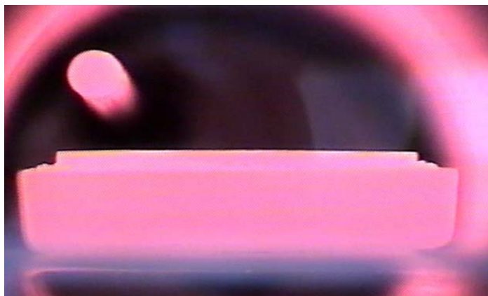
Figure 6: \text{Na}_2\text{CO}_3 drop on mullite specimen after melting
