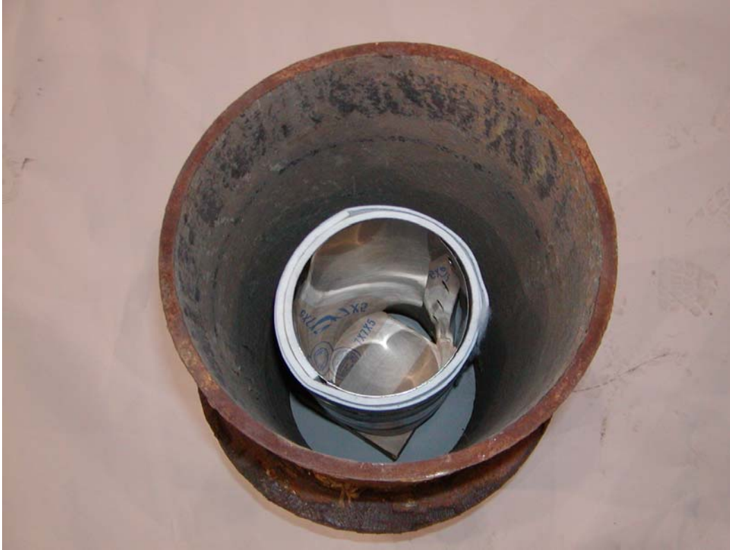
Figure 7. Unset Patch Inside 12" CI Bell and Spigot Joint
