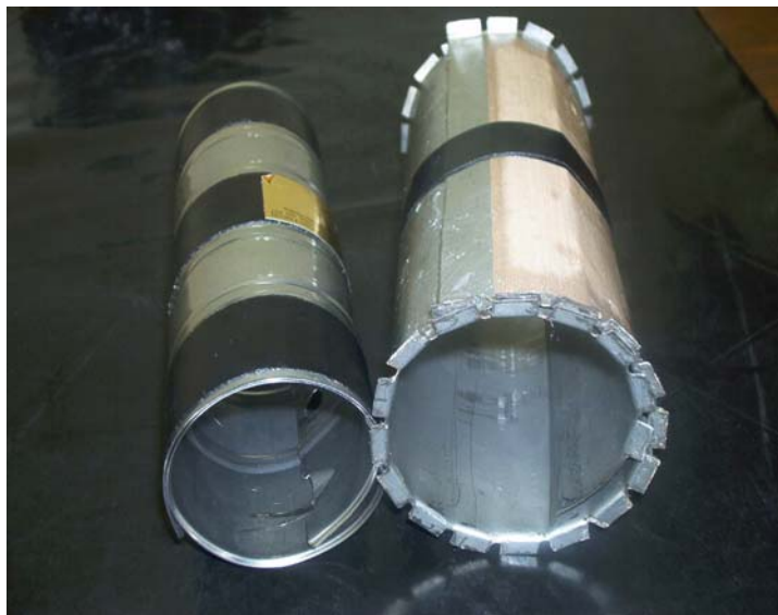
Figure 5. Coiled Diameter Comparison for 28 and 24 Gage
