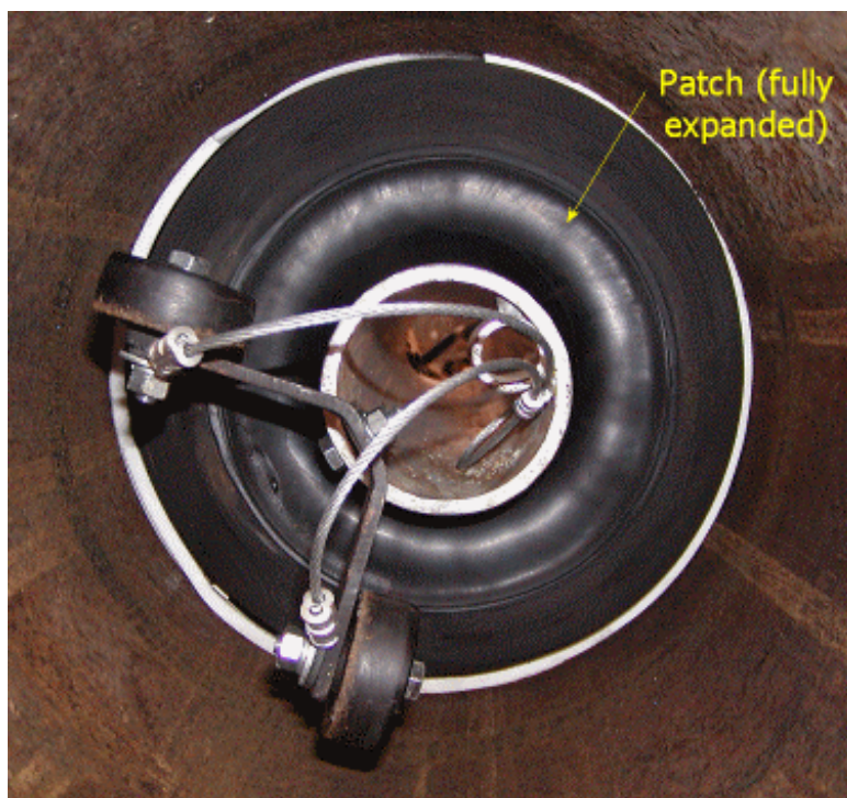
Figure 9. Patch Setting Test
