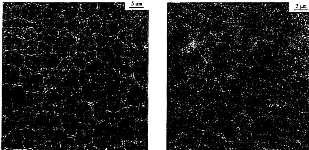
Figure 1. AFM micrographs that reveal the polycrystalline microstructure formed via spontaneous nucleation and growth of solids in supercooled liquid matrix: (left) 200 nm Al on SiO<sub>2</sub>, and (right) 100 nm Cu on Ta coated (7 nm) SiO<sub>2</sub>.
