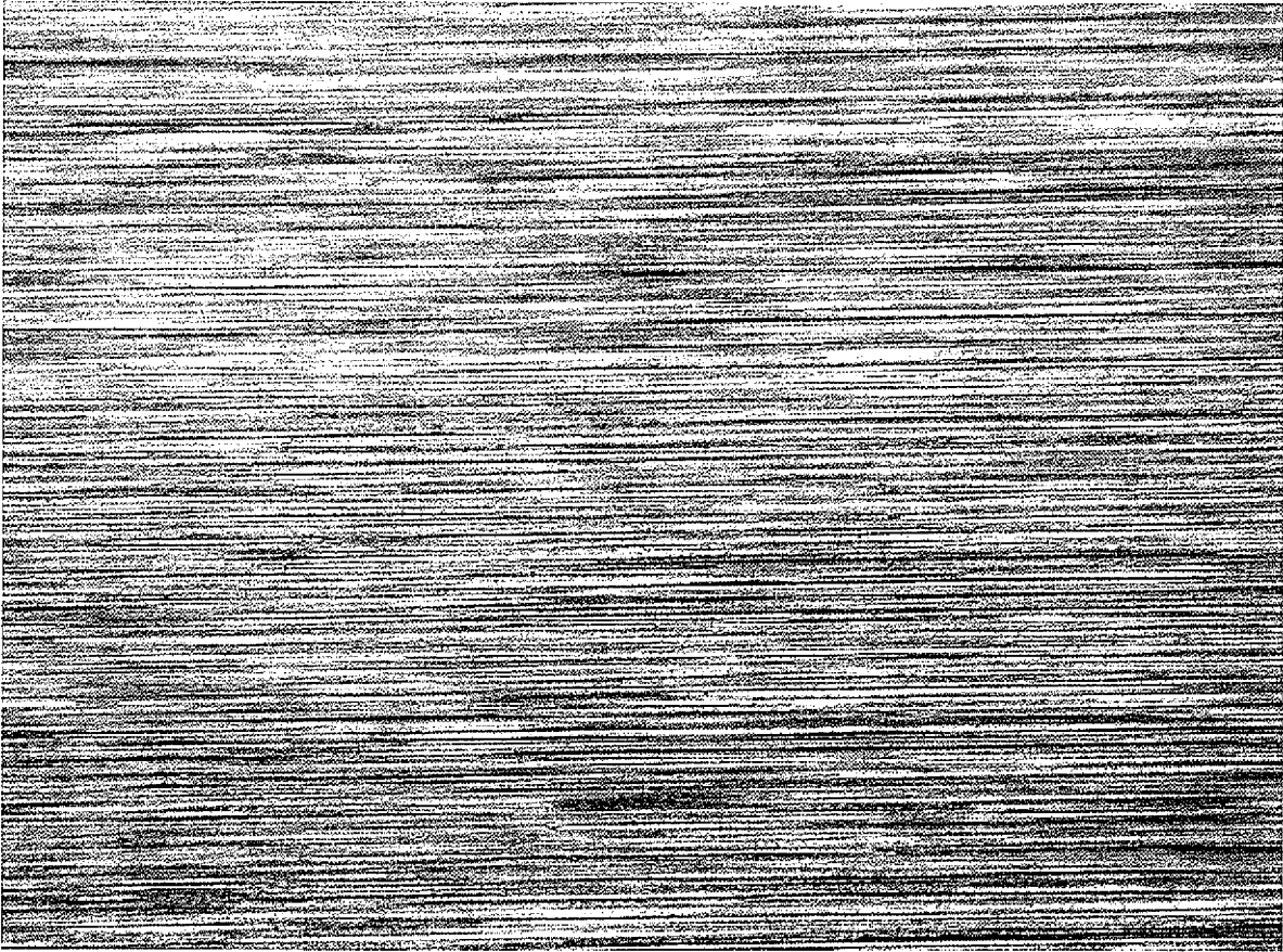
Figure 2. Digital Image of a laboratory specimen prepared using a grinding process, at 25x magnification under fluorescent lighting.
