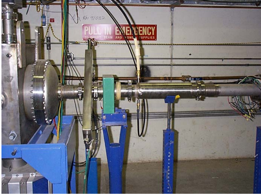
Figure 10. The downstream end of the Chopper. A small wide-aperture vertical pulsed dipole could be placed just after the Chopper, followed by a horizontal pulsed dipole as shown in figure 8. A new arrangement of the wire scanner, Pearson transformer and Griffin monitor will provide the needed space.
