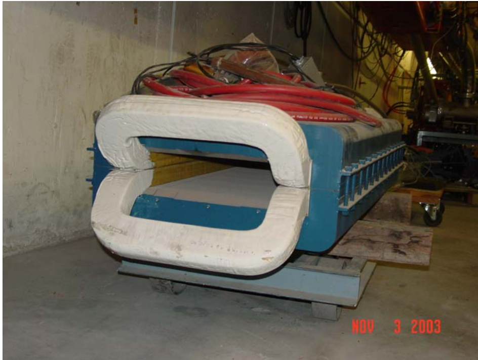
Figure 6. Cooling Ring Dipole magnet in storage, showing 12-inch gap width. The magnet characteristics are described in TM-0777.
