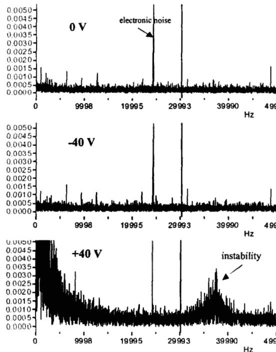
In other experiments (November to December, 2000), a second electrode, a 2 cm diameter circular disk (paddle) probe is placed in the center of the plasma. A bias voltage is applied to the paddle probe to draw an axial current. Once again, the instability appears in the plasma. Now, by adjusting the bias voltages on the cylindrical (rotation) electrode and the disk (paddle) electrode, it is possible to maintain control over the growth and formation of this instability.
