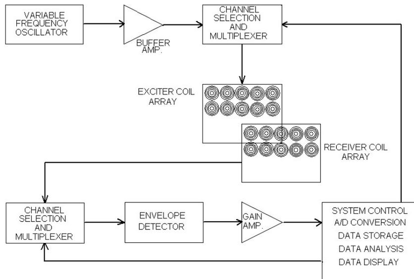
Figure 2. Data acquisition hardware schematic
