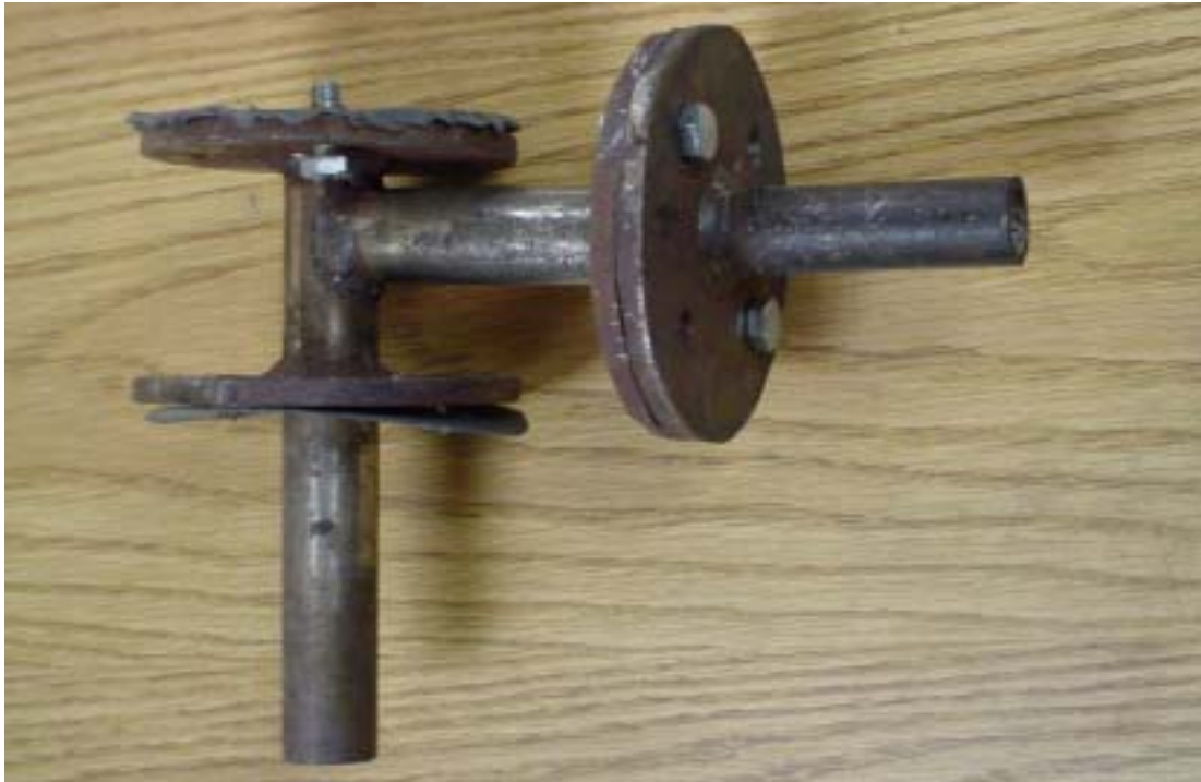
Figure 32. The Thermocouple Probe (K-Type ) for Gasifier Simulator (Hot Model)
