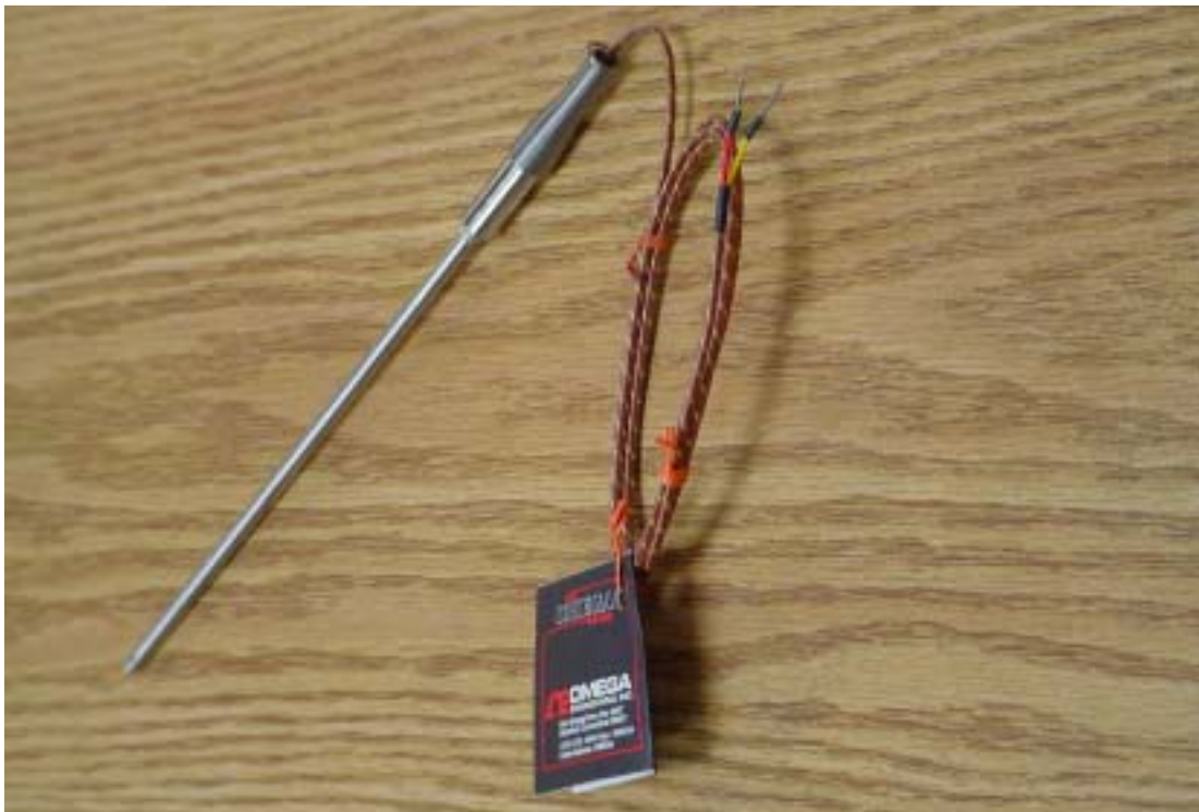
Figure 32. The Thermocouple Probe (K-Type ) for Gasifier Simulator (Hot Model)
