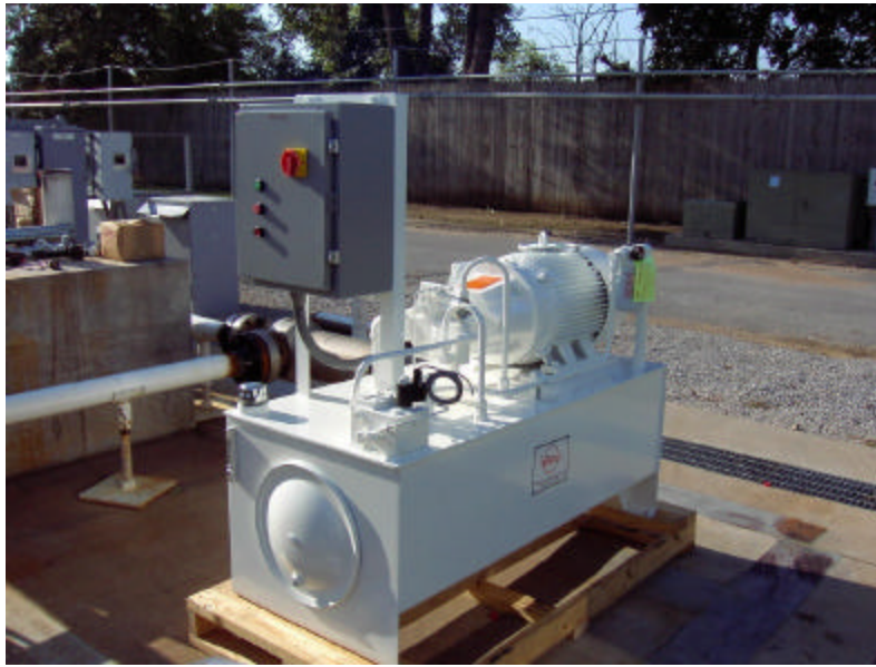
Figure 3.10 - New Hydraulic Power Unit to Rotate Pipe
