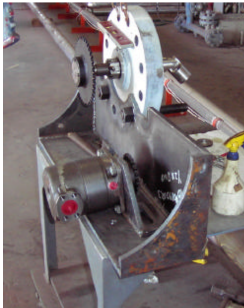
Figure 3.9 – Components of Drive System to Rotate Pipe
