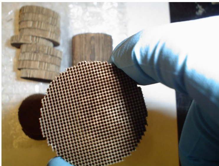
Figure 3: Autothermal reforming catalyst sections
