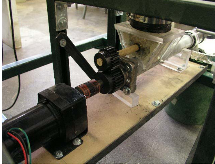
Figure 2. Bottom feeder, hopper, and agitator assembly.
