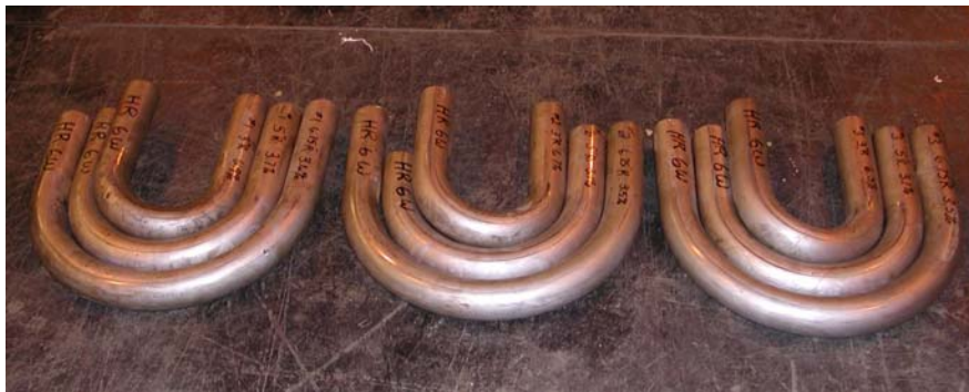
DIGITAL IMAGE SHOWING U-BENDS OF HR6W TUBING WITH STRAINS OF 15%, 20% AND 35%.
