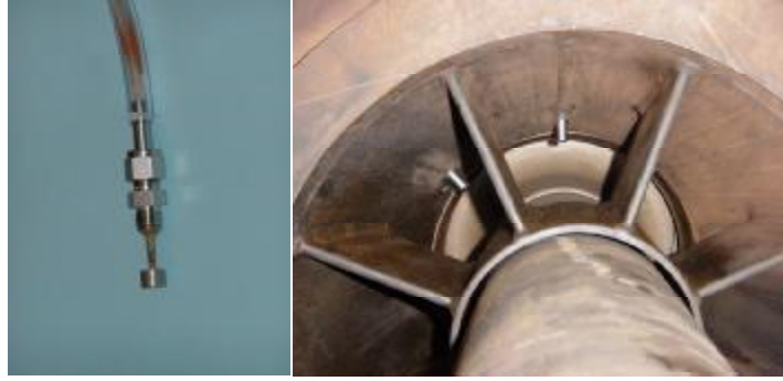
Figure 11. Photographs of a Small Typical Laboratory Surge Sensor Drag Probe and the Installation of Two Surge Sensor Probes in Field Compressor Ready for Testing.
