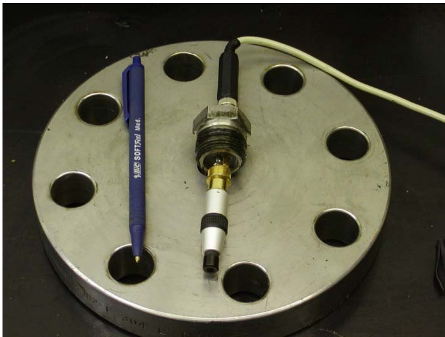
Figure 5 – Model 3031 microphone installed in 3/4" high pressure feed-through
