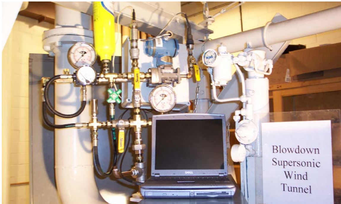
Figure 1 - WVU 2 nd Generation Portable Acoustic Monitoring Package (PAMP) for Natural Gas Transmission Pipelines at Pressures up to 1000 psi.
