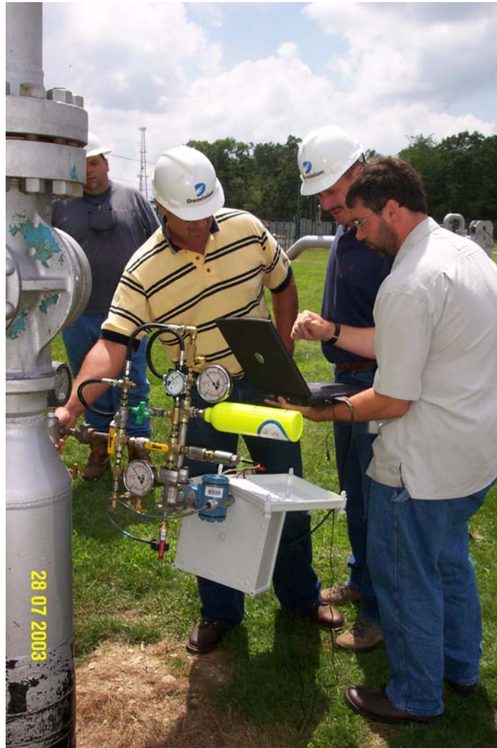
Figure 14 – PAMP installed on transmission line at Dominion Transmissions North Summit storage facility
