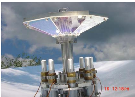
Fig. 27: Secondary mirror and fiber array
