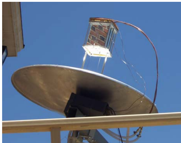
Fig. 4: Cooling circuit and thermocouples on top of NI tube
