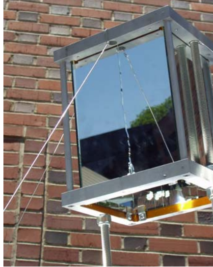
Fig. 3: Non-Imaging Device with broken mirror
