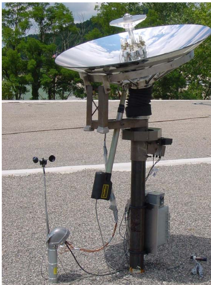
Fig. 28: Solar tracker-collector assembly
