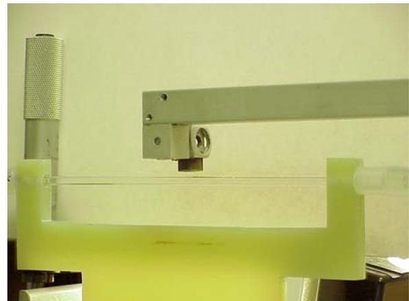
Figure 22. (a) Experimental apparatus for studying magnetic particle liquid-suspension behavior under influence of magnetic fields. (b) Glass, square flow channel (2mm x 2mm) showing external magnet positioned above the channel.
