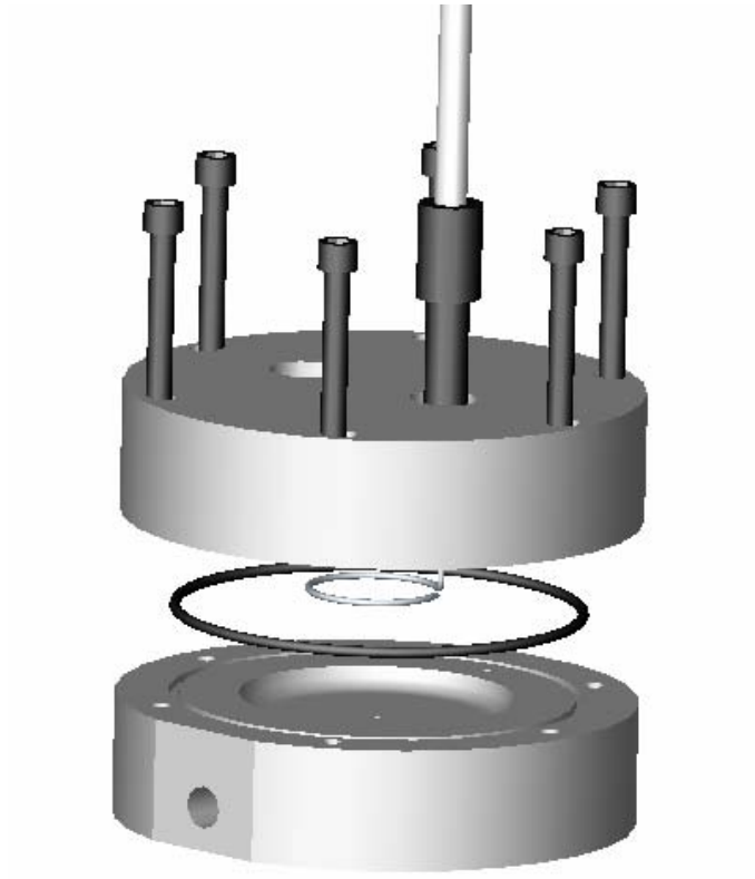
Figure 5. Exploded view of Engine Cylinder Test chamber assembly, shown with circular ring electrode
