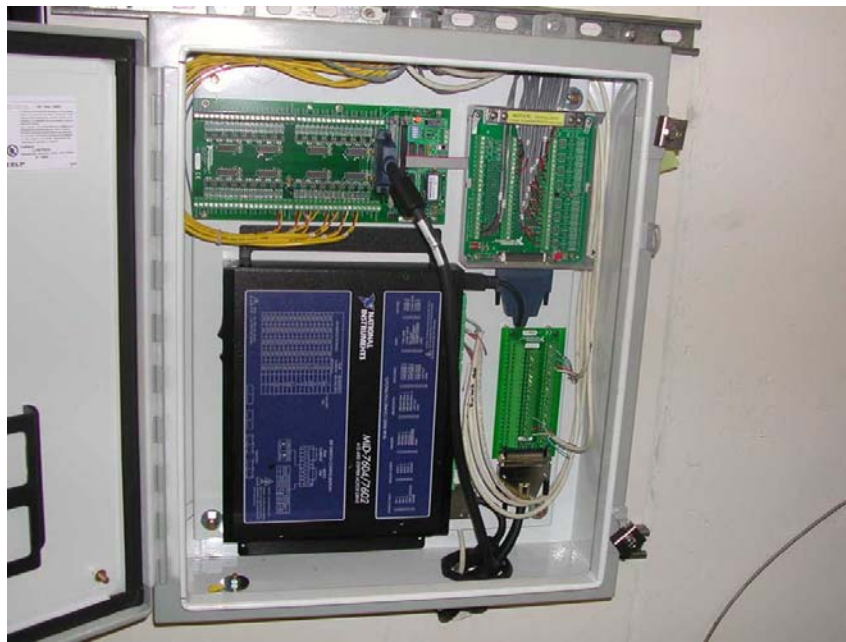
Figure 7. Main panel for data acquisition and control equipment. Top left AMUX-64T, top right SCB-68, bottom left MID-7604, bottom right CB68-LPR
