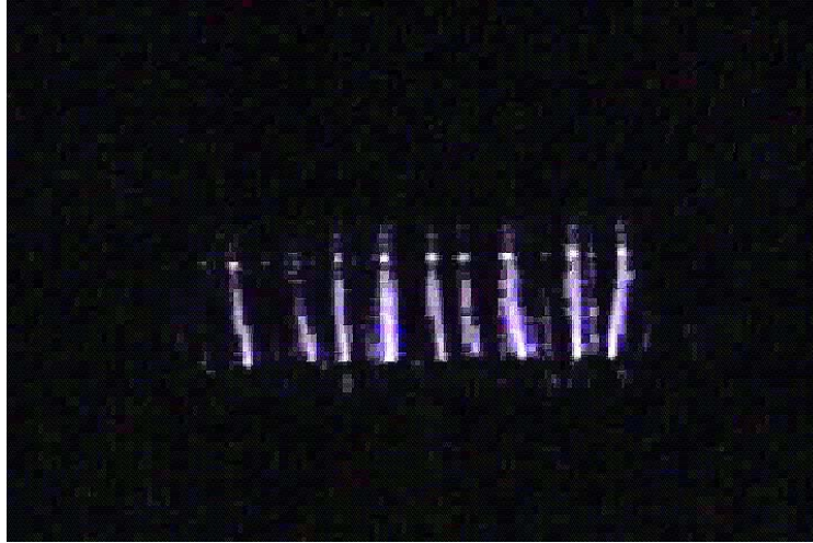
Figure 10. Photograph of corona discharge in engine cylinder test chamber with open top plate installed. .5mm diameter electrode 50mm circular ring
