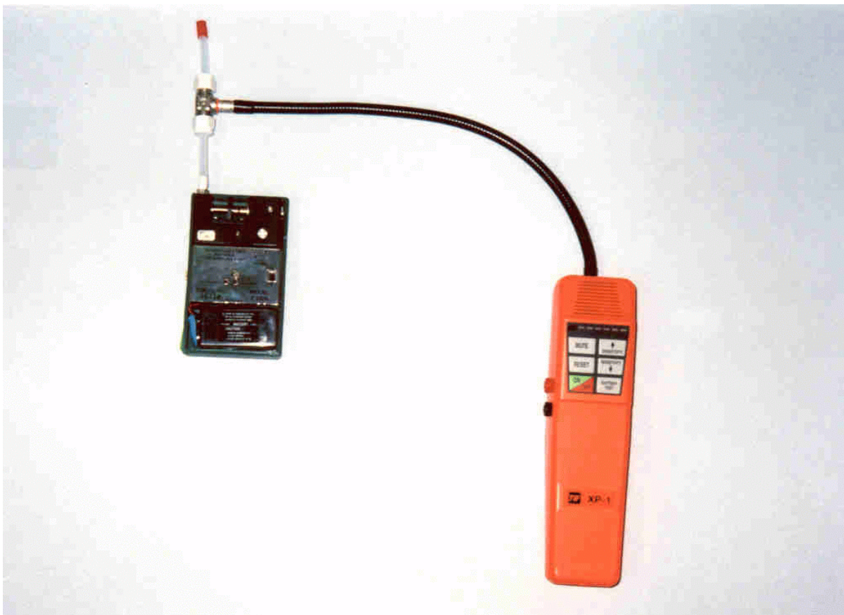
Figure 12. TIF XP-1 Leak Detector with Auxiliary Du Pont P200A Personal Sampling Pump
