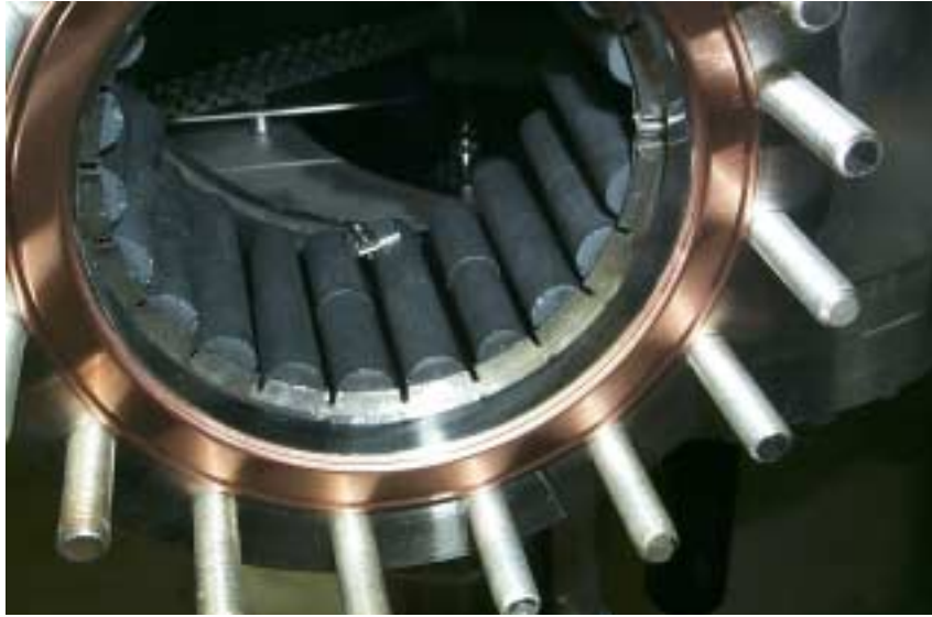
Figure 1: (color) Photo showing ferrite rods placed at the entrance or exit of the flying-wire cavity. This circular opening will be joined to the usual 3.806'' \times 1.75'' Recycler Ring beam pipe.
