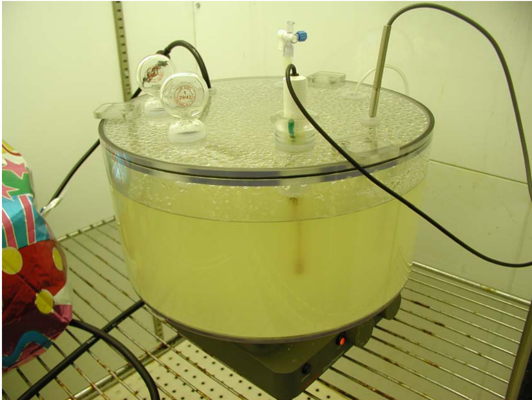
Fig.1. Experimental vessel equipped with temperature and pH probes, sampling ports (with 3-way stopcock) and mylar argon reservoir. Note the turbidity of the media due to a high cell density.
