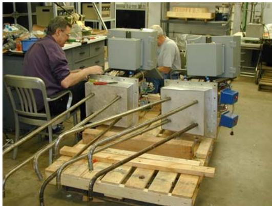
Figure 1. Air heater tube testing assemblies during final installation of instruments and controls
