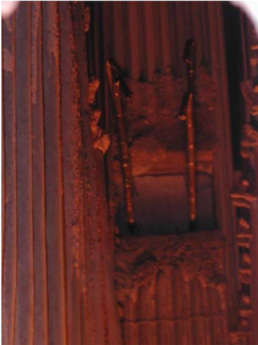
Figure 3. Air heater tube testing assembly installed in the upper
