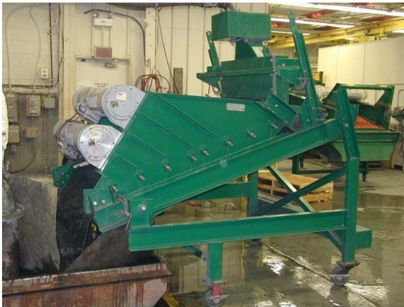
Figure 4: Derrick's Stack Sizer test machine used to carry out commercial testing of the sample of secondary mill feed. Six different scenarios were tested.
