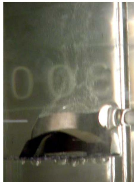
Figure 6. Dissolution in 3M HNO<sub>3</sub>
