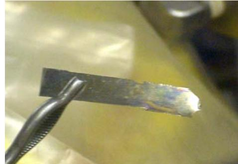
Figure 4. Stripped Uranium Metal
