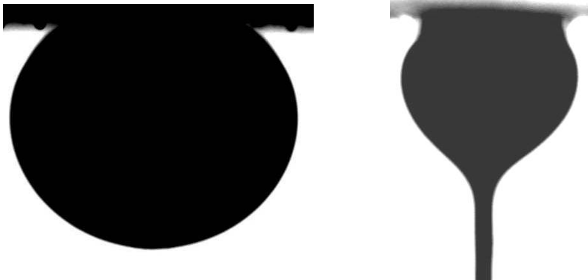
Fig. 3 – Receding and advancing angles of the sessile oil droplet in contact with the calcite plate before aging with crude oil.
