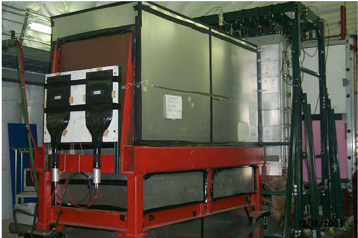
Figure 6: The hadron calorimeter (left) and electromagnetic calorimeter (right) in the beam line at the Meson Laboratory, ready for final testing with beam.
