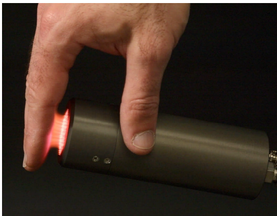
Fig. 1. Plasma source (Atomflow 250 TM ) operating with helium and nitrogen at 10 W/cm 2 [33].
