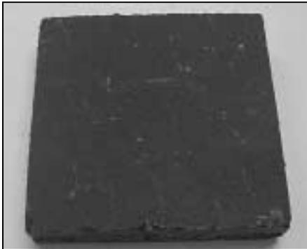
**Figure 3. Sample tile with resin mass fraction of 12% (No phase change material)**
