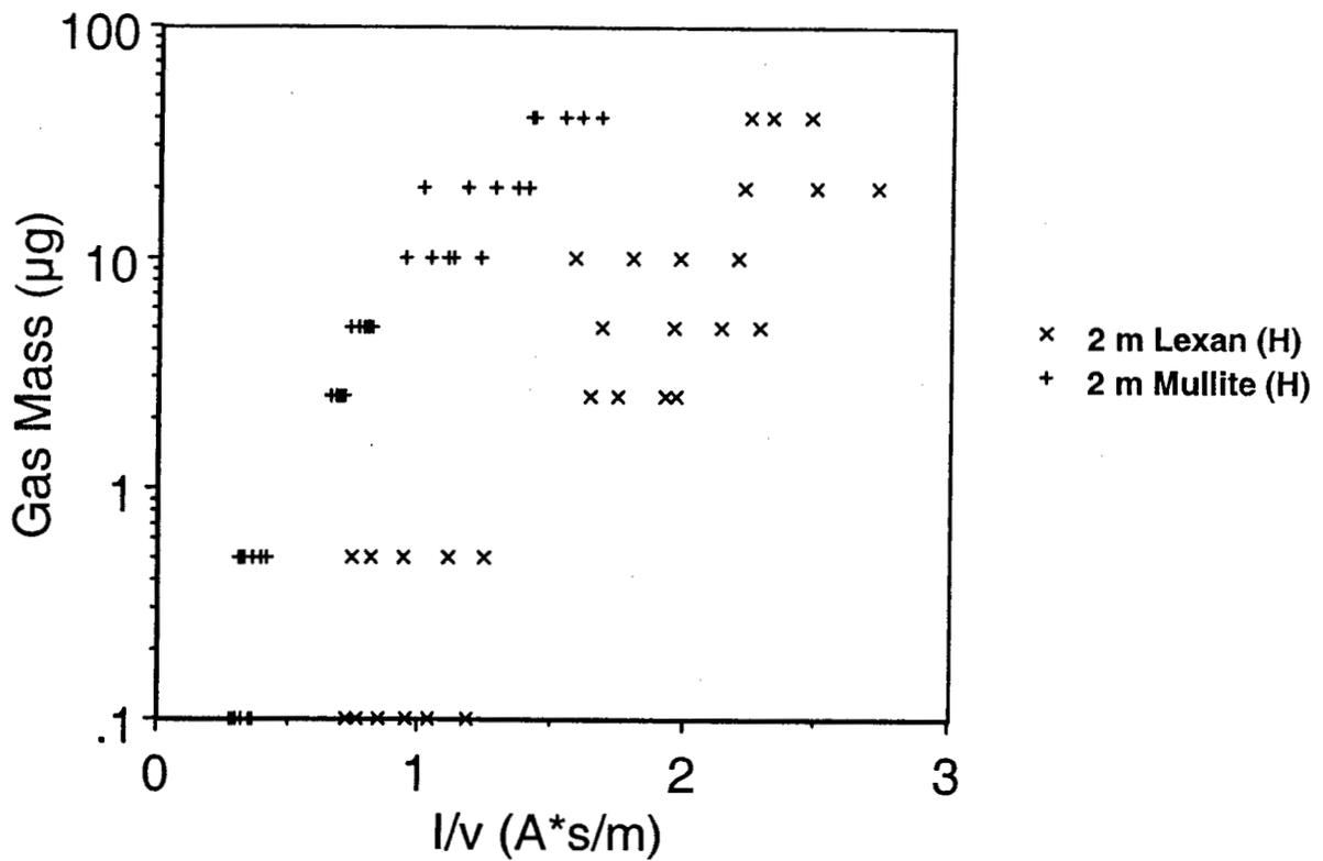
Hydrogen gas mass vs.  $I/v$  on 2 m gun
