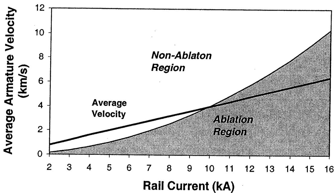
Figure 5.1 The threshold current for ablation
