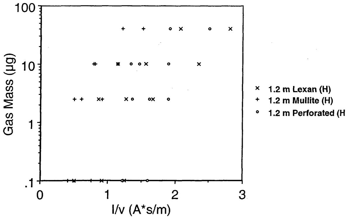
Hydrogen gas mass vs. I/v on 1.2 m gun
