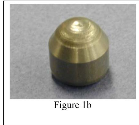
Figure 1. Two Views of the Round Top Drill Bit Insert. The insert is typical of the cutting tools placed on rotary drill bits. (Orientation of the fibrous monolith was right to left, from the round top to the flat base.)
