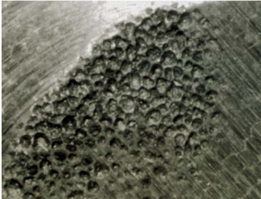
Figure 3. Close-up of the Hammer Induced Damage to the Bottom of the Insert. The damage appears to mostly occur in each fibrous monolith cell. Compare the damaged to the undamaged cells.
