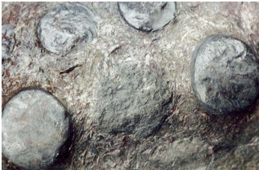
Figure 6. Highly Worn FM Insert on a Worn Superior Rock Bit Drill Bit. Compare the worn insert (center) to the surrounding current art inserts. The two current art inserts at the top exhibit brittle failures. The test insert has similar FM failures as exhibited by the hammer tests in Figure 3.
