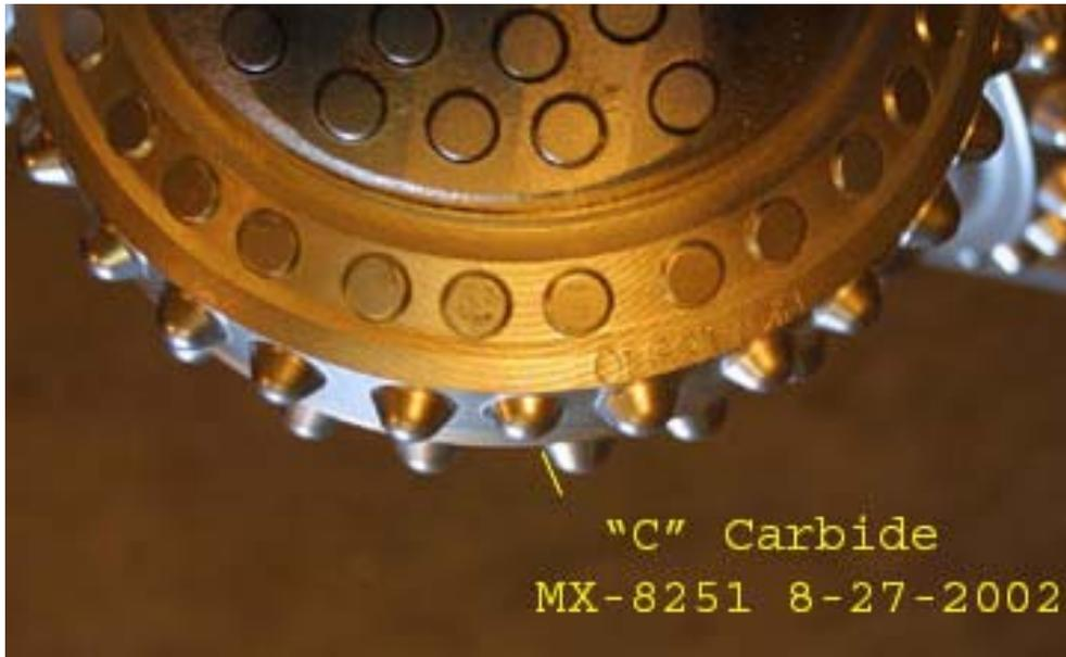
Figure 4. Drill Bit Used in Field Tests. The Superior Rock Bit test bit was 16.5 inches in diameter. The “C” carbide was the new art test insert.
