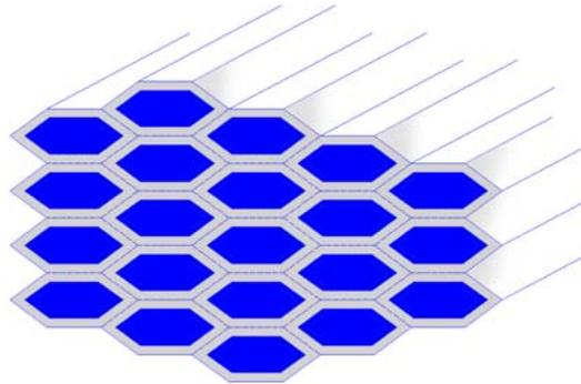
Figure 2. Schematic Drawing of the Core and Boundary Areas in a Fibrous Monolith. The test inserts were composed of a tungsten carbide core (blue, 96 % carbide) and a cobalt boundary (gray, 100% cobalt).
