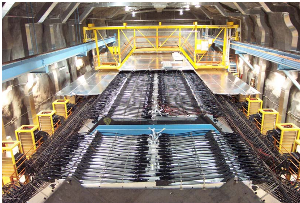
Figure 3. Photograph of the top of the MINOS far detector at Soudan. This August photo shows the nearly completed veto shield covering the top of Supermodule 1 and also the first few planes of Supermodule 2. The veto shield is used to flag the presence of cosmic ray tracks that can create a background to atmospheric neutrino events in the detector. A clean sample of muon-neutrino charged-current events is being used to search for any difference in the oscillations of atmospheric neutrino and antineutrino events, which would constitute a violation of CPT symmetry.
