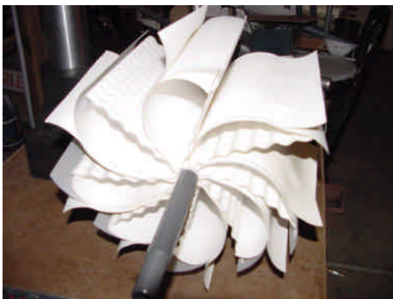
Plate 10. Continuous Membrane Pack Affixed to the Permeate Tube
