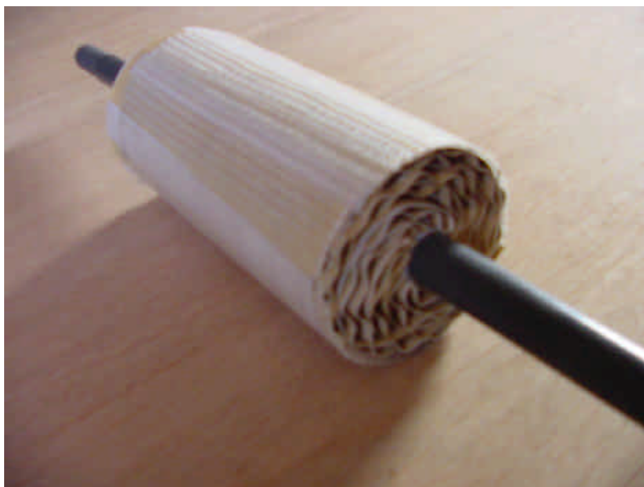
Plate 11. Membrane Pack Inserted into the Sleeve
