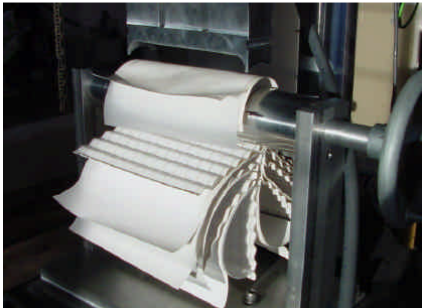
Plate 8. Connecting Eight Fluted leaves by Forming Circular Leaves
