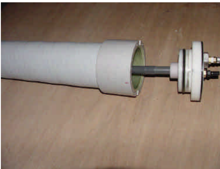
Plate 6. Membrane Housing used in Integrity Tests
