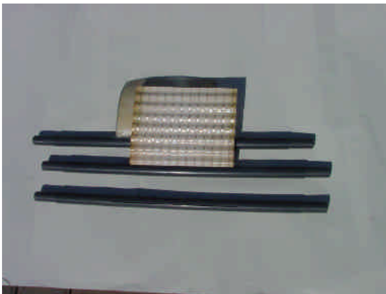
Plate 5. Membrane Leaves Prepared for Integrity Testing
