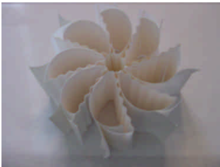
Plate 9. Continuous Membrane Pack Formed by Eight Fluted Leaves Interconnected through Eight Circular Leaves
