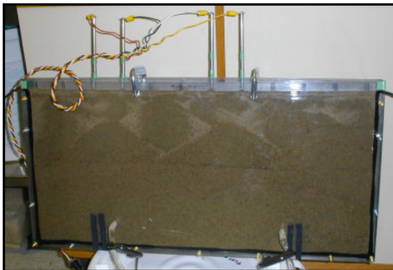
Figure 12: Photograph of bench-scale 2-D resistivity apparatus ‘ant farm’. A lexan box approximately 58cm by 28cm by 1.5cm contained a soil sample with known heterogeneities. Standard 4-wire IP dipole-dipole array measurements were made using the laboratory electronics system. After correction of the raw measurements to account for the true 2-D nature of the apparatus, IP imaging was performed using the RES2DINV software.
