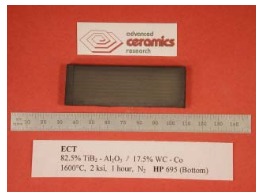
82.5% \text{TiB}_2 - \text{Al}_2\text{O}_3 / 17.5% WC-Co
