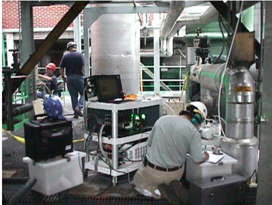
The photo shows the test surrounding at the Eastman incinerator facility. The PI took notes next to the prototype ABFLIP unit. Two Eastman staff were present at the far back of the photo.
