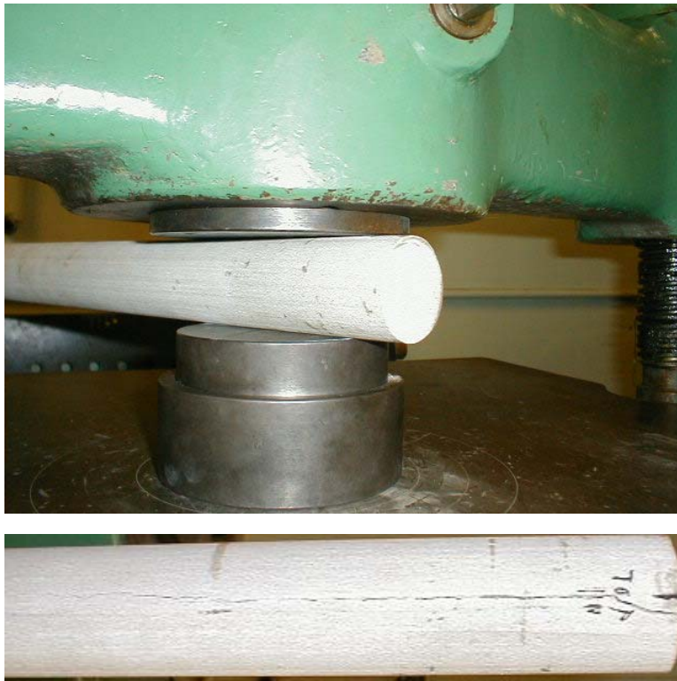
Figure 3: A Layered Berea rock being fracture using the modified Brazilian procedure.
