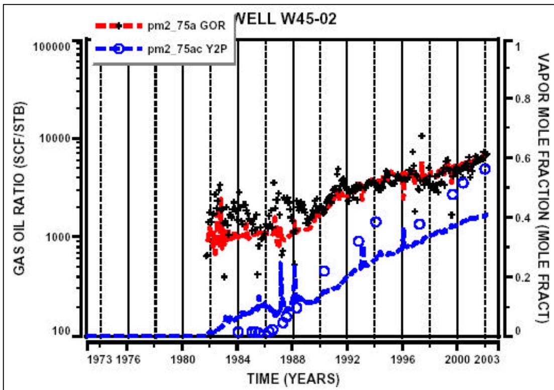
Figure 6. Simulation history match plots for EBU 45-2. The upper plot is the match from the original pilot model; the lower plot is from the current model. “Y2P” is the nitrogen content of produced gas. Symbols are field data; lines are model data.
