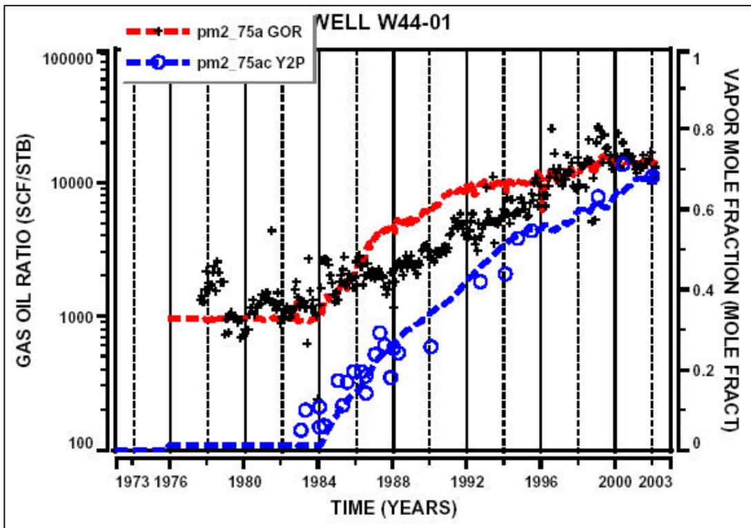
Figure 5. Simulation history match plots for EBU 44-1. The upper plot is the match from the original pilot model; the lower plot is from the current model. “Y2P” is the nitrogen content of produced gas. Symbols are field data; lines are model data.
