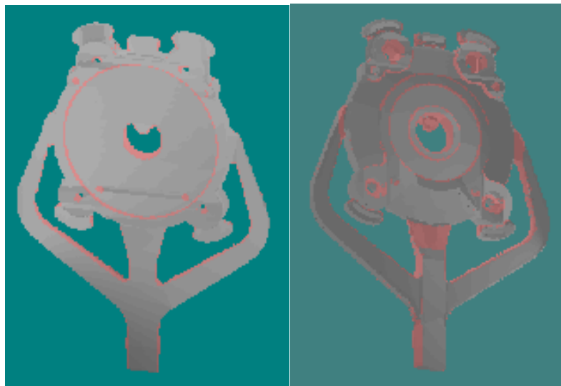
(a) The photograph of the ejection marks obtained from the real casting product.
