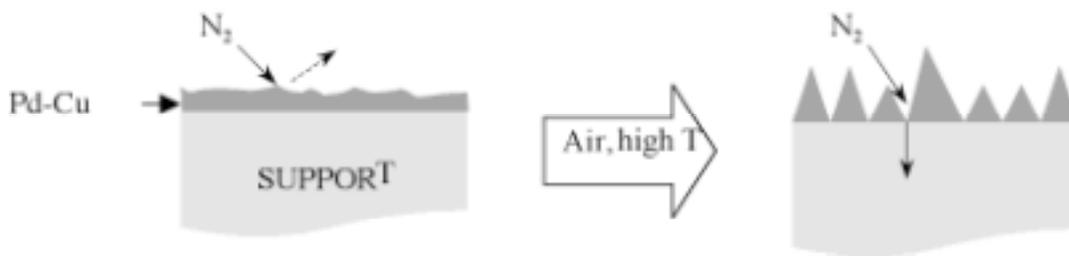
Figure 8. Cartoon showing our hypothesis for mechanism of air purge on thin Pd alloy membranes.
