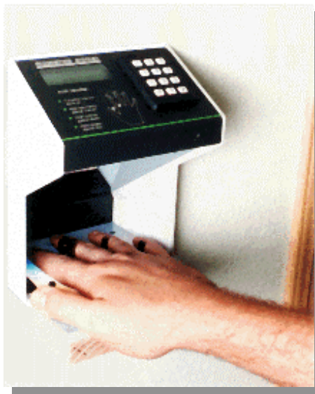
Figure 11: Access Control Device Using Hand Geometry For Identification
