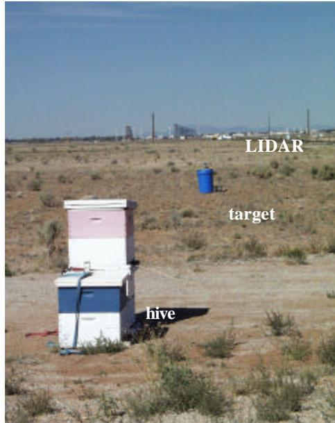
**Figure 4: Photo that illustrates the near-linear relationship between the hive, target, and the LIDAR system, and also illustrates shows the distance between the LIDAR and the targets.**
