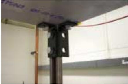
Figure 7: a bolted joint of the test structure
