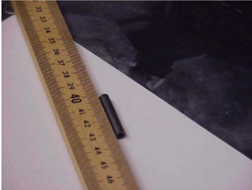
Fig. 5 Sintered tube of  $\text{La}_{0.6}\text{Sr}_{0.4}\text{Fe}_{0.8}\text{Co}_{0.2}\text{O}_{3-x}$  for use in isotopic transient measurements.
