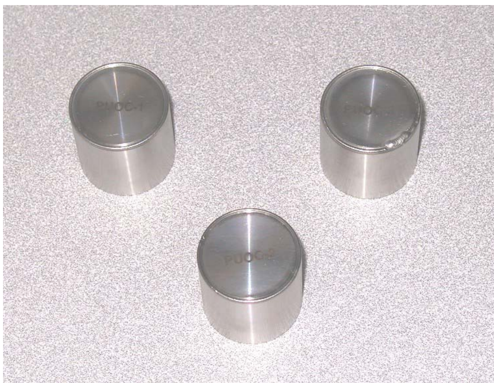
Figure 4. Set C (of the five sets) of encapsulated plutonium oxide standards is pictured. The outer diameter and height of each capsule is 3.2 and 4.2 cm, respectively. The identification numbers were etched onto the individual capsule parts prior to assembly and welding.
