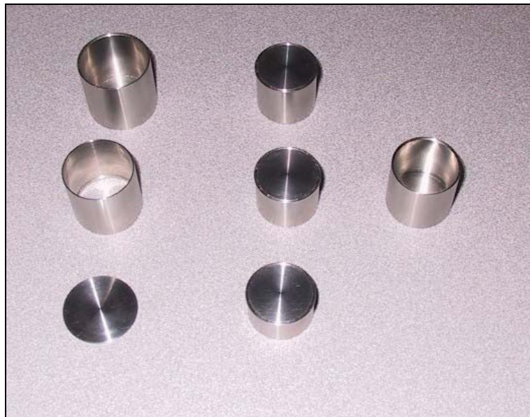
Figure 6. Photograph of stainless steel capsule parts. The “inner can” is at the right. Its “lid” is one of the three “retaining cylinders” (center). The “outer can” and its “centering ring” and “lid” (top to bottom) are at the left.
