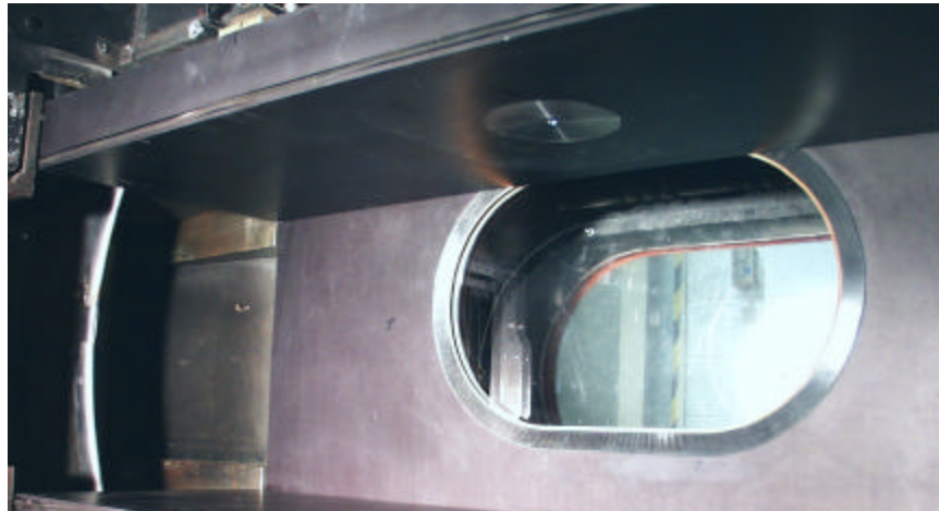
Figure 4: The jet nozzle hardware installed into the wind tunnel's top-wall mounting position. Both views are seen from the front of the wind tunnel with an open test section; (a) shows the wind tunnel support structure and the jet above the tunnel wall; (b) shows the interior top wall of the test section.
