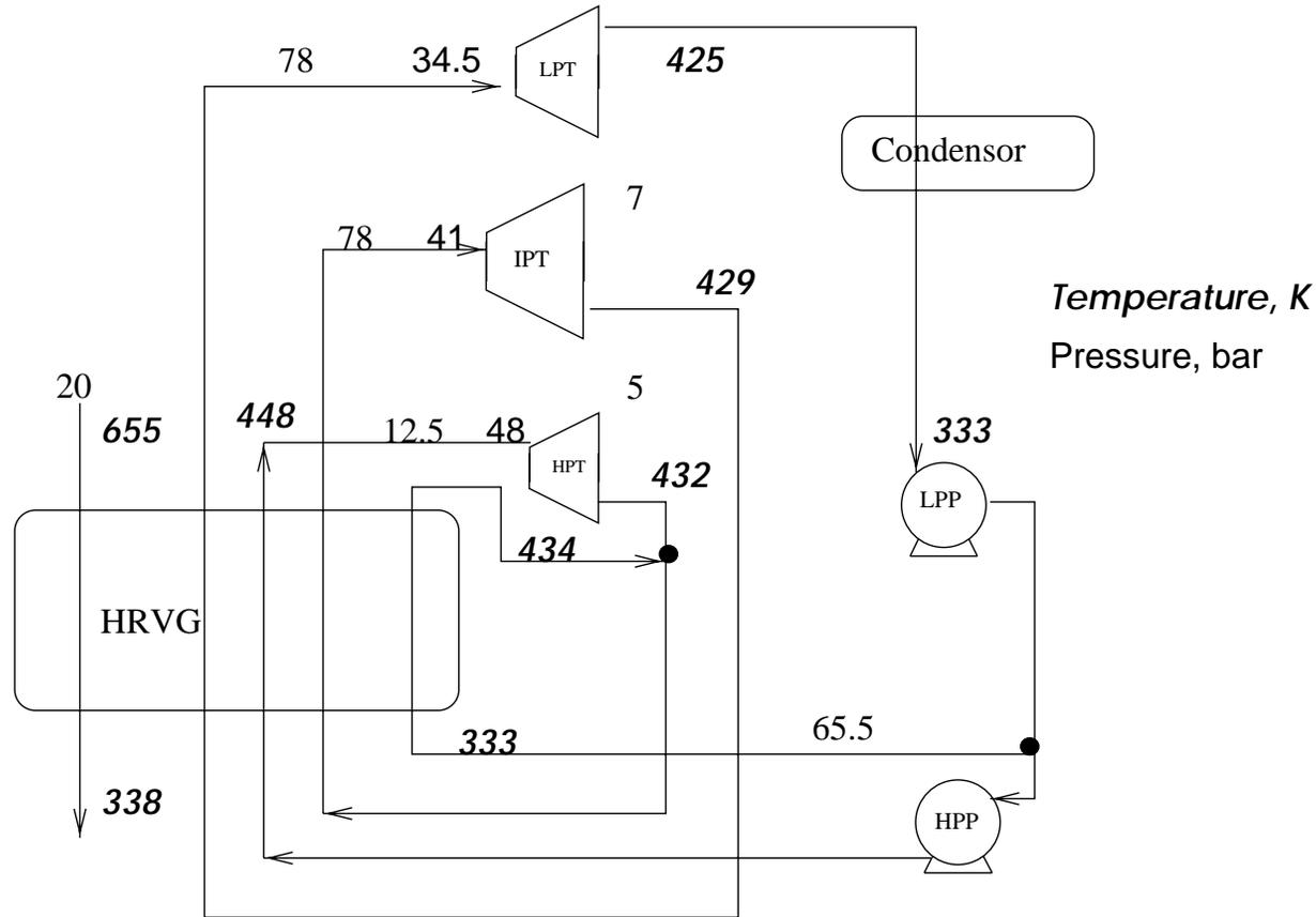
Optimal cycle using 90% ammonia working fluid. Profit= \$19M/yr
